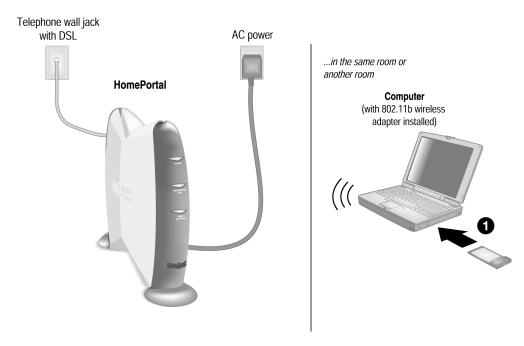
**Note:** If you use a 2Wire wireless adapter (PC card or USB adapter) for wireless networking, the HomePortal Setup Wizard software automatically configures it to communicate with the HomePortal during setup, but you will need to install the driver. See Appendix A for detailed installation instructions.
